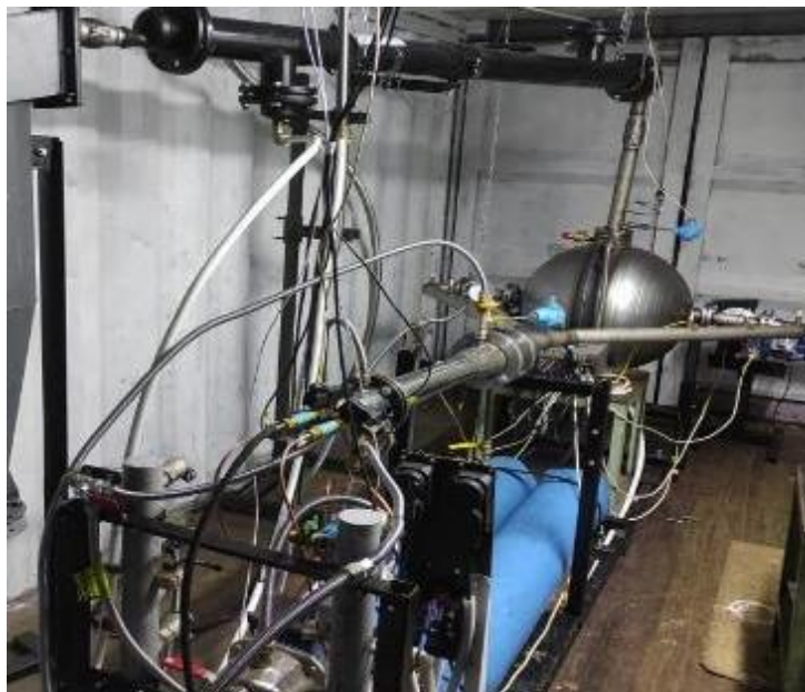
Fig. 4. Photograph of a mobile organic waste converter in a 20-foot sea container [7].
