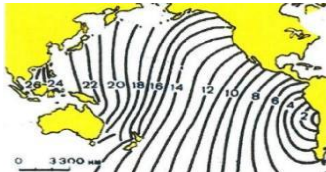
Fig. 3. An initial state of the sequential propagation of the Chilean tsunami of May 22, 1962, obtained with the help of ENM, is given.
